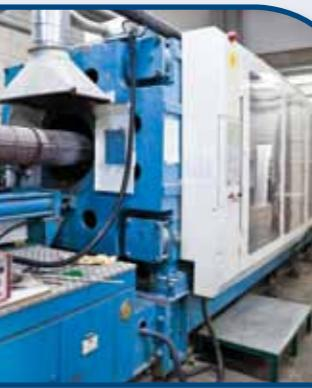
CNC Automated Injection machines production line for plastic parts, capable of producing parts weighting from 10 gr up to 6.5 kgr.
