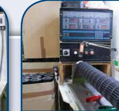
Ultrasonic welding machines for plastic fans production and fan balancing machines for precise parts production.
