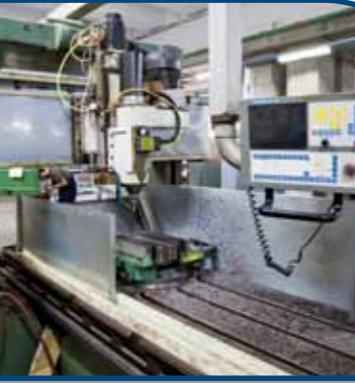
PRO Engineer Software station for MOULD design connected with a 4 AXIS CNC mill with a long up to 3 meters table for big Moulds production.
